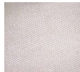
8330 Meta-Aramid Mesh Weight: 100-106g/m 2 Width: 198-203cm
